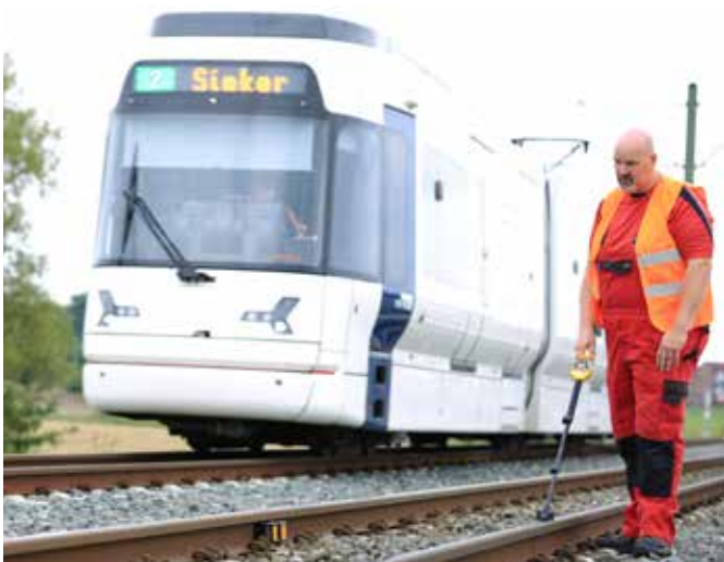
ISKO device for locating insulation and contact faults for trouble-shooting short circuits and contact resistance in the track
