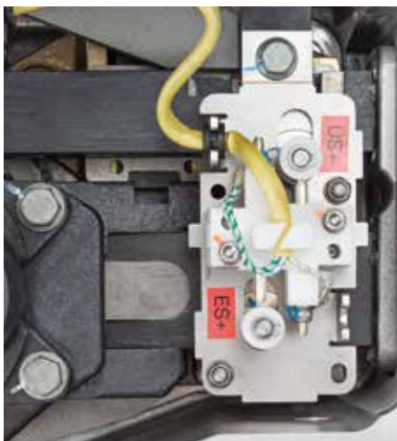
End-position monitoring with clearly visible forced-guided contacts
