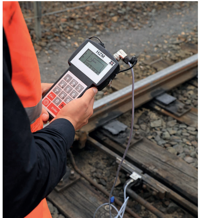
The HZM force-measuring device for force testing on point machines
