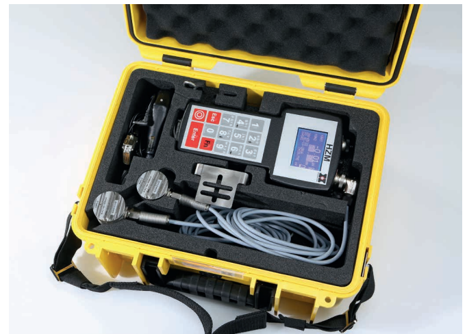
Example: HZM force-measuring device set
