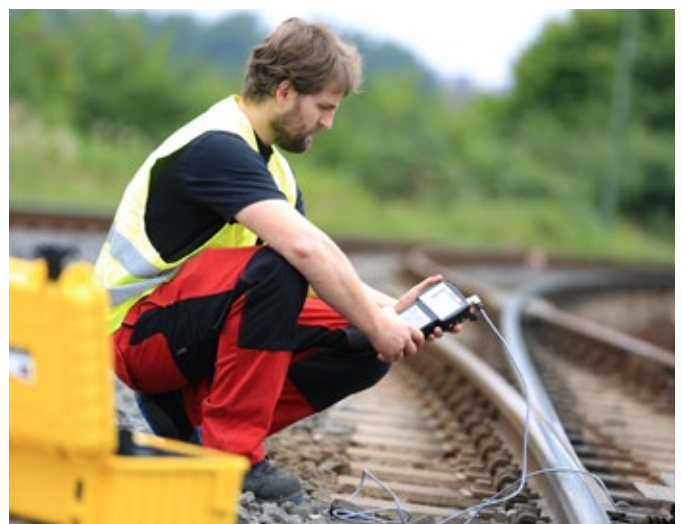
Force-measuring device HZM in operation
